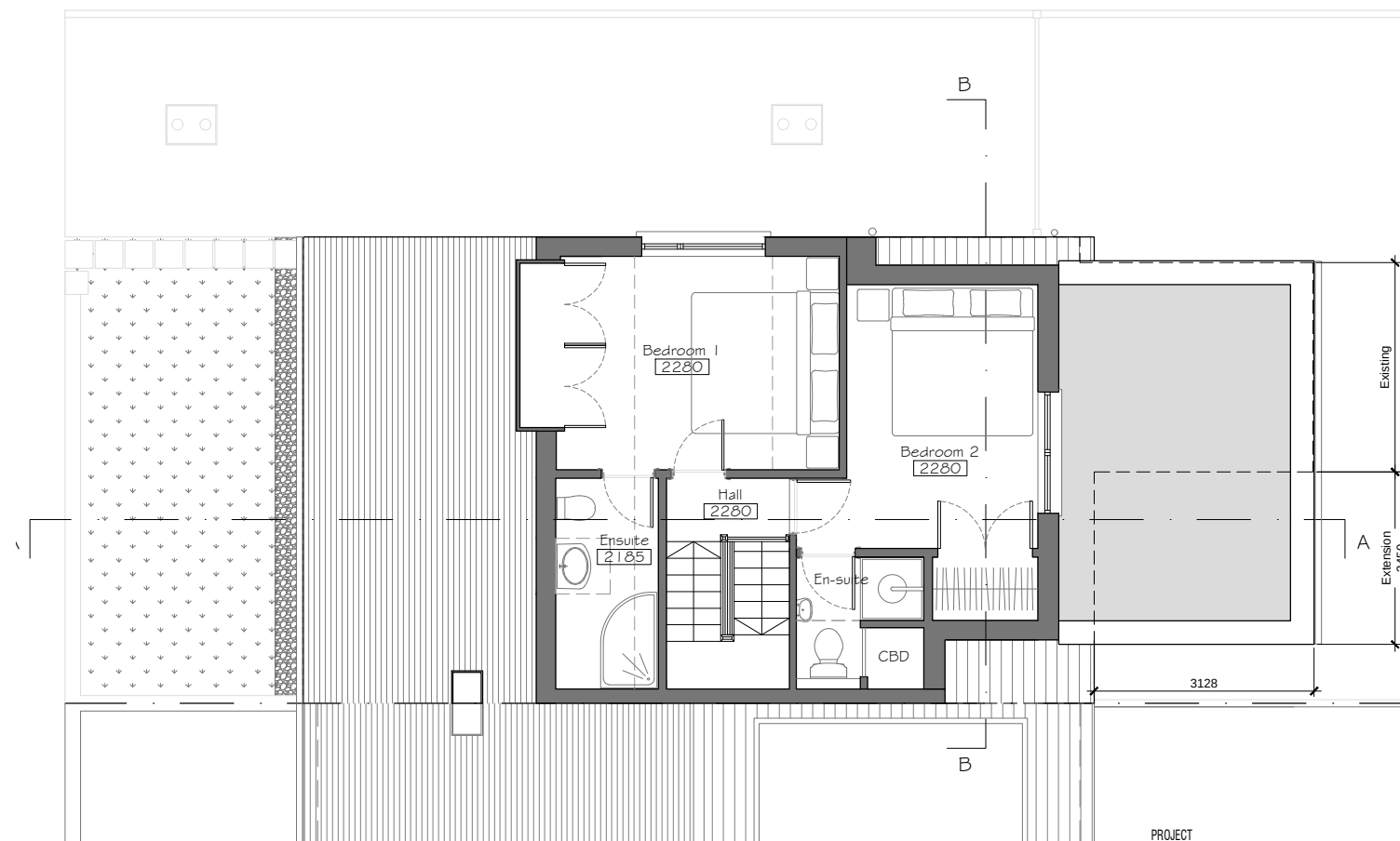
Proposed First Floor Plan Scale 1:100
