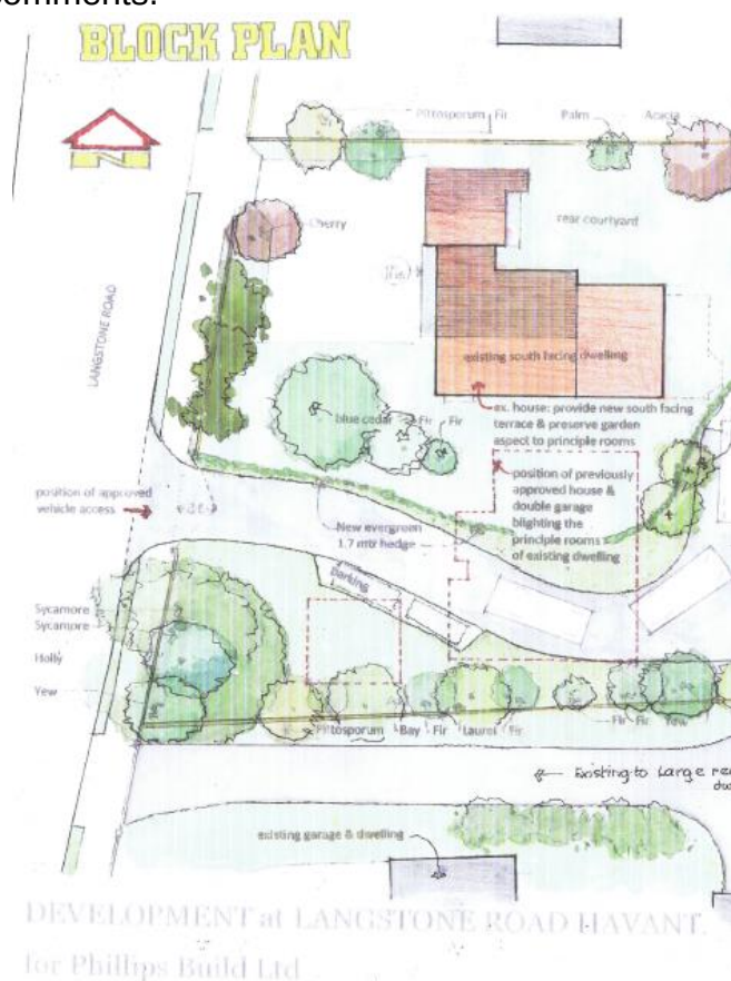
Fig 3 Partial site plan of current proposal showing a meandering driveway (heavily landscaped) to lessen any undue impact on the street scene
