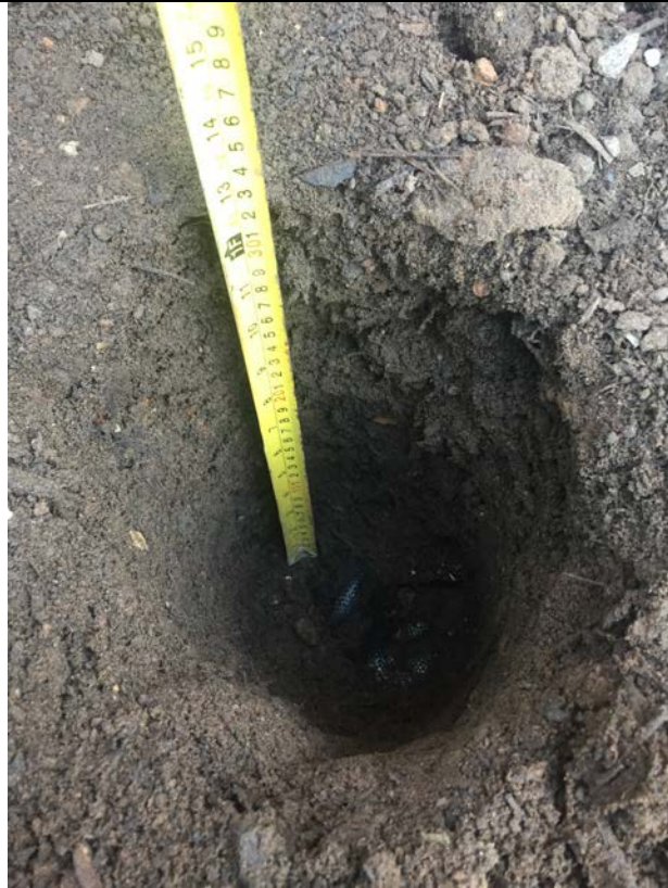
HP301 showing emplacement of black membrane at 300mm bgl.
