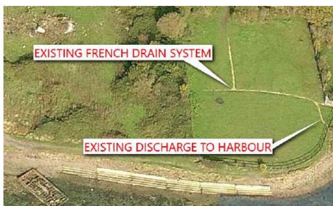
Fig 3.5.2 – Aerial Photograph showing French drain
