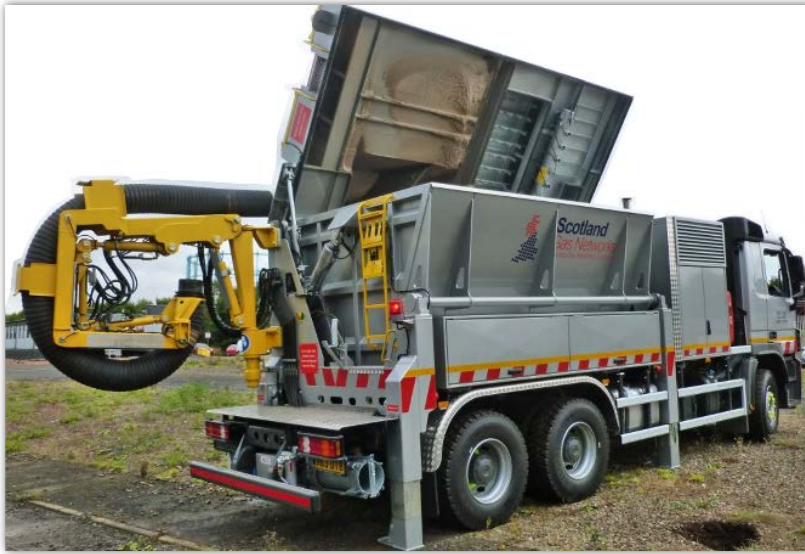
Figure 17. Large Vacuum Excavator
