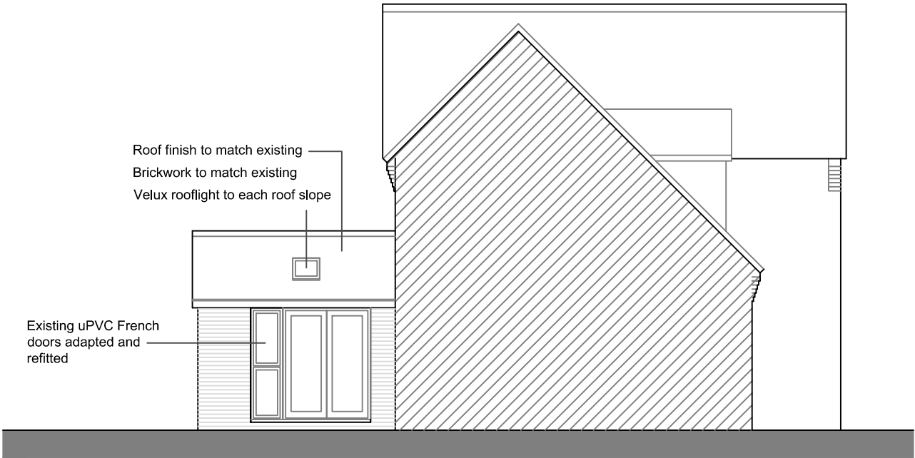
PROPOSED Side elevation Scale 1:100
