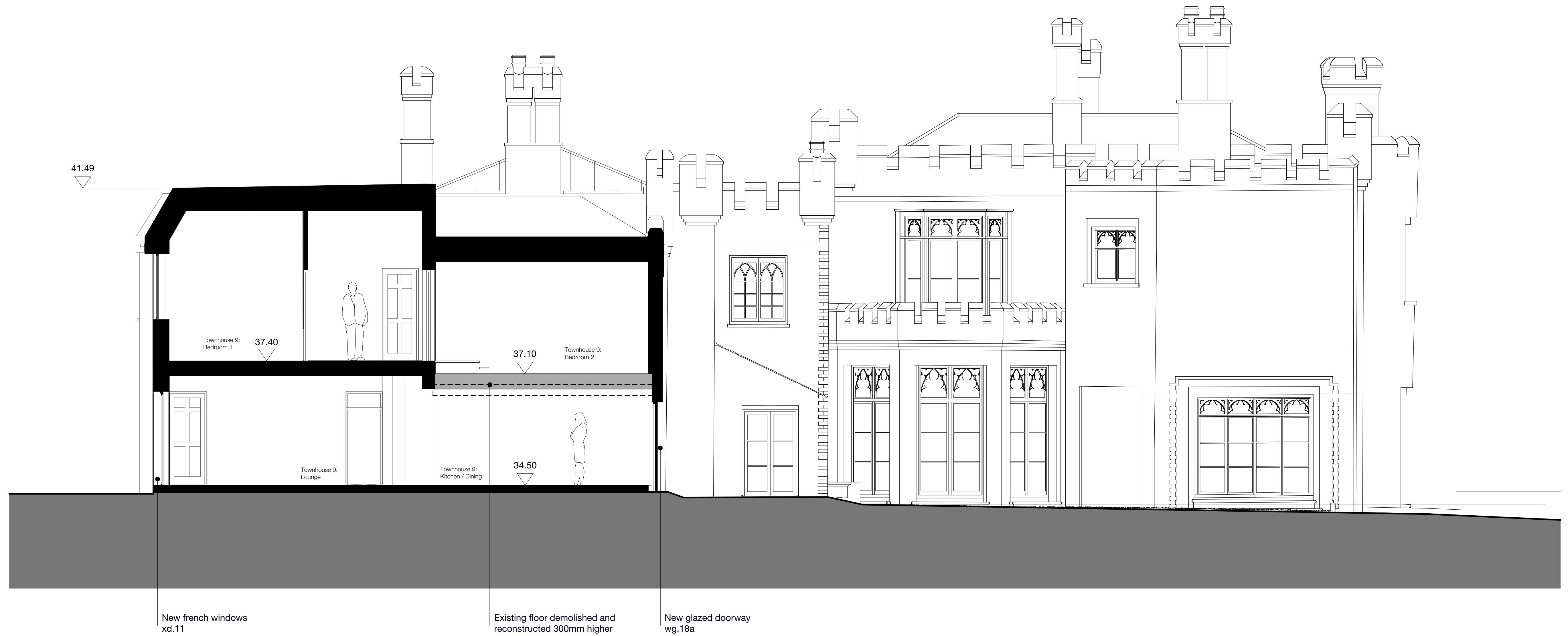
7 Main House - Proposed Section A-A SCALE: 1:50
