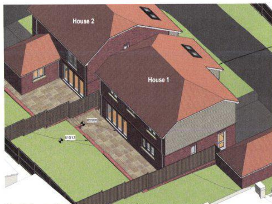
Retaining walls to rear of houses 1 & 2
