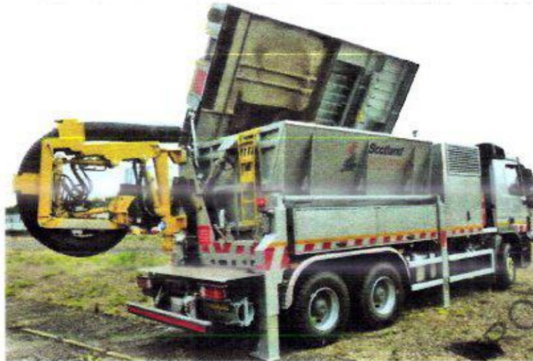
Figure 17. Large Vacuum Excavator
