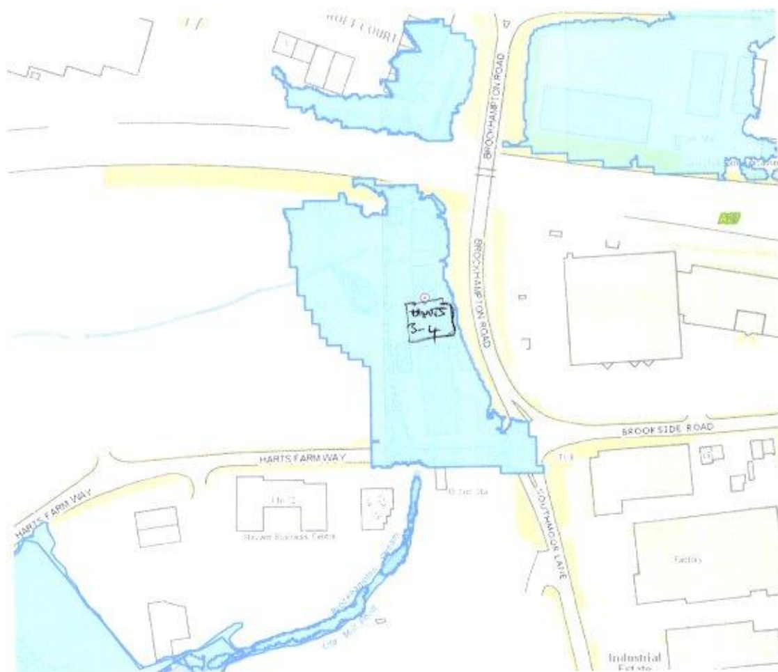
Flood zone 2 identified – 3-4 Premier Buildings, Brockhampton Road
