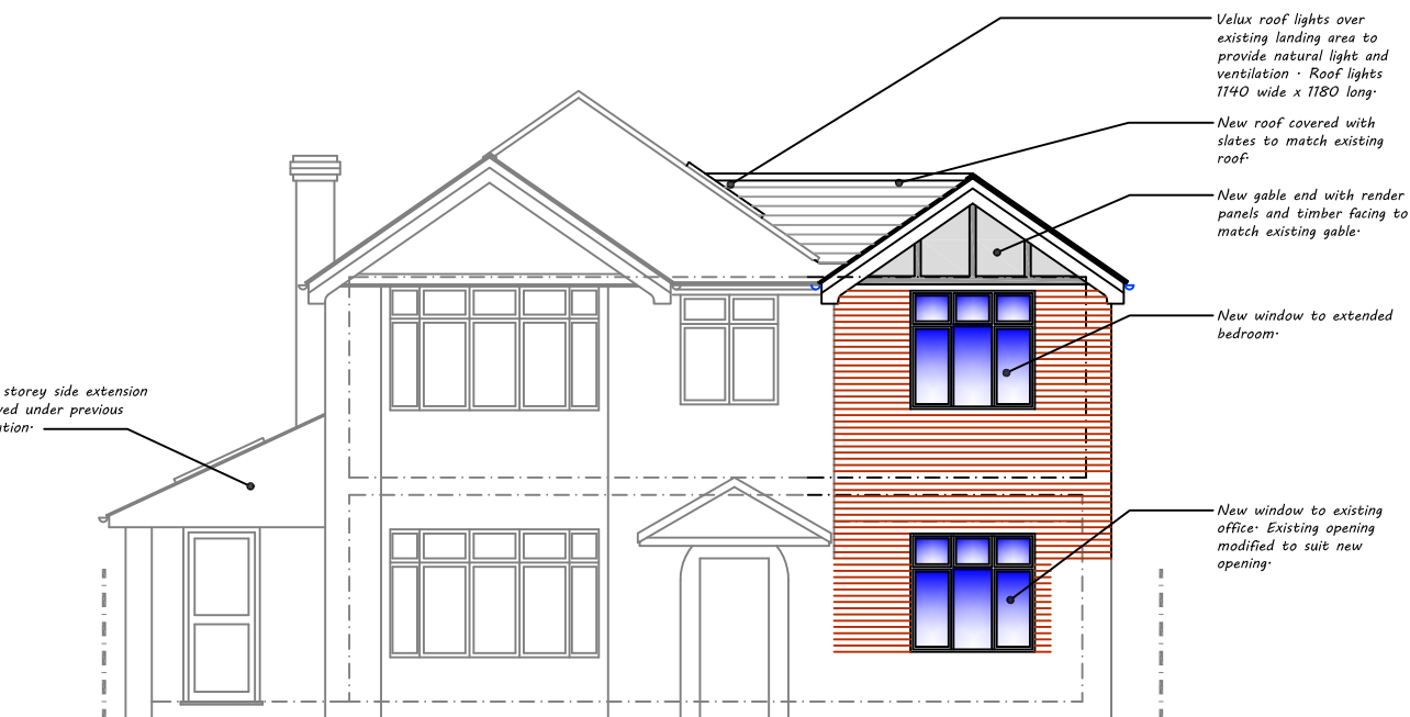
Front Elevation as originally applied for
