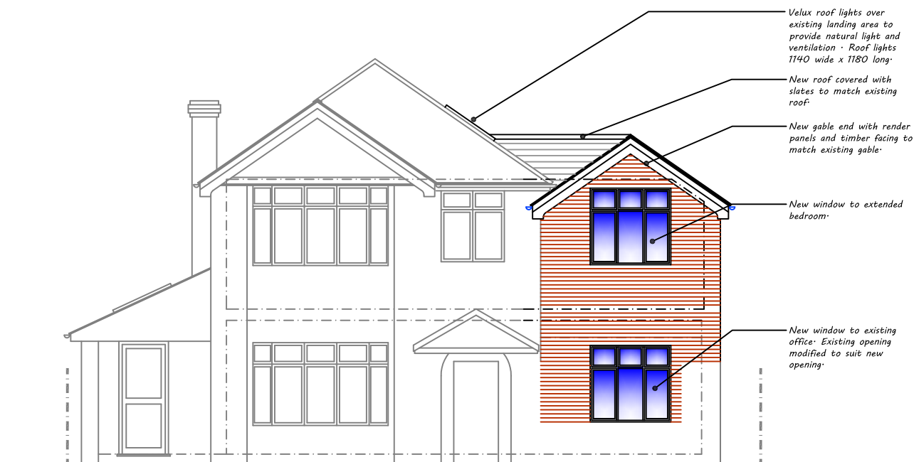
Front Elevation - Current application
