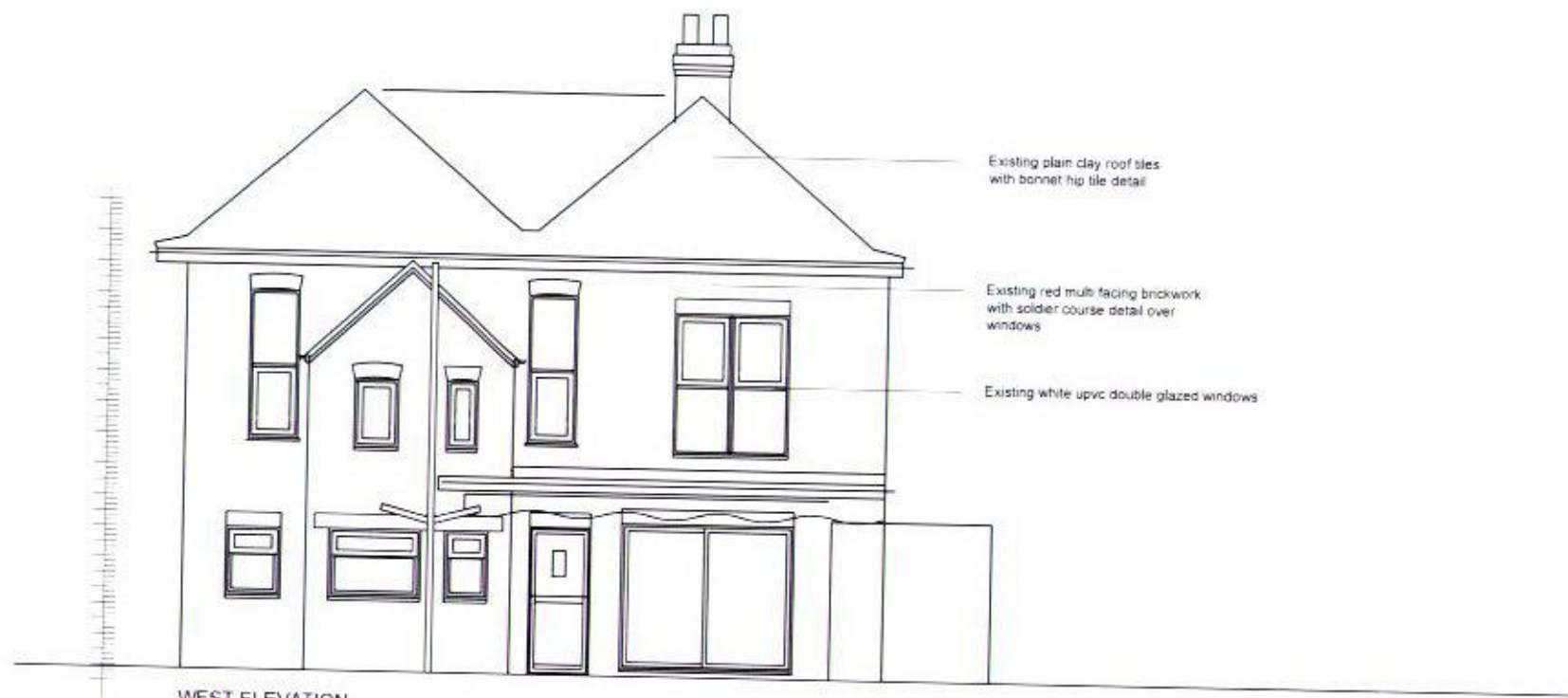
WEST ELEVATION EXISTING
