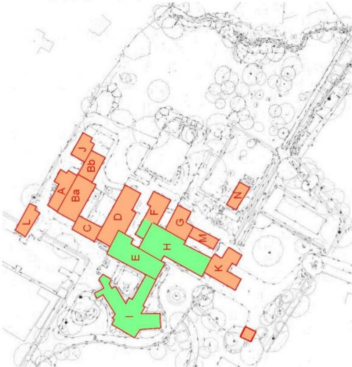
Figure B.1.2.1. Location of destructive search/ inspection works (highlighted in orange) and retained buildings (highlighted in green).
