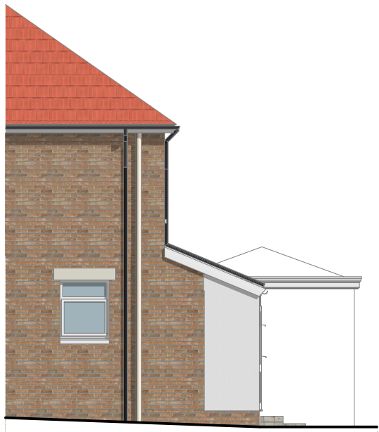
Existing Side Elevation 1:100
