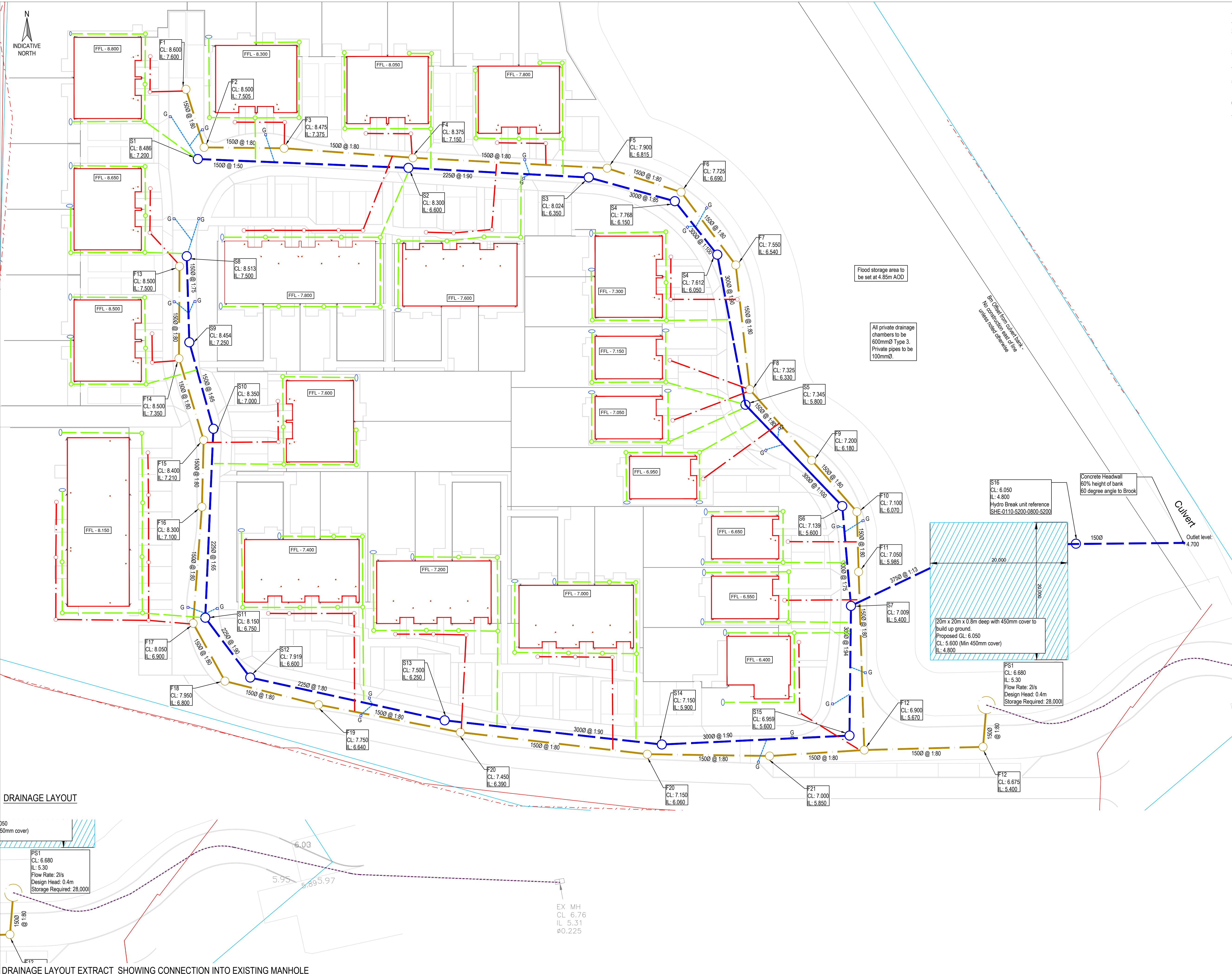
DRAINAGE LAYOUT EXTRACT SHOWING CONNECTION INTO EXISTING MANHOLE
