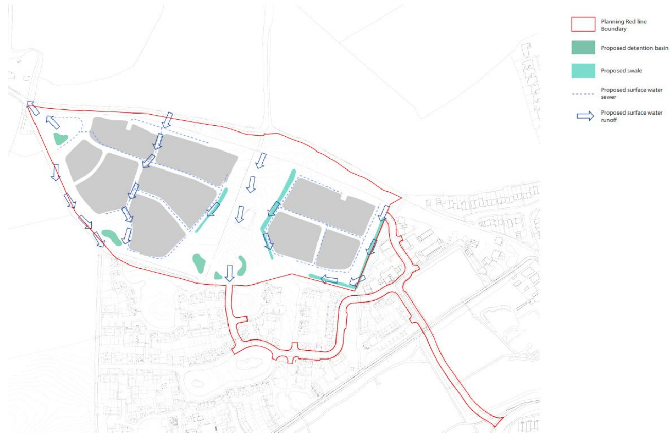
Figure 9 Illustrative diagram detailing the drainage and flood risk strategy of the proposed development.
