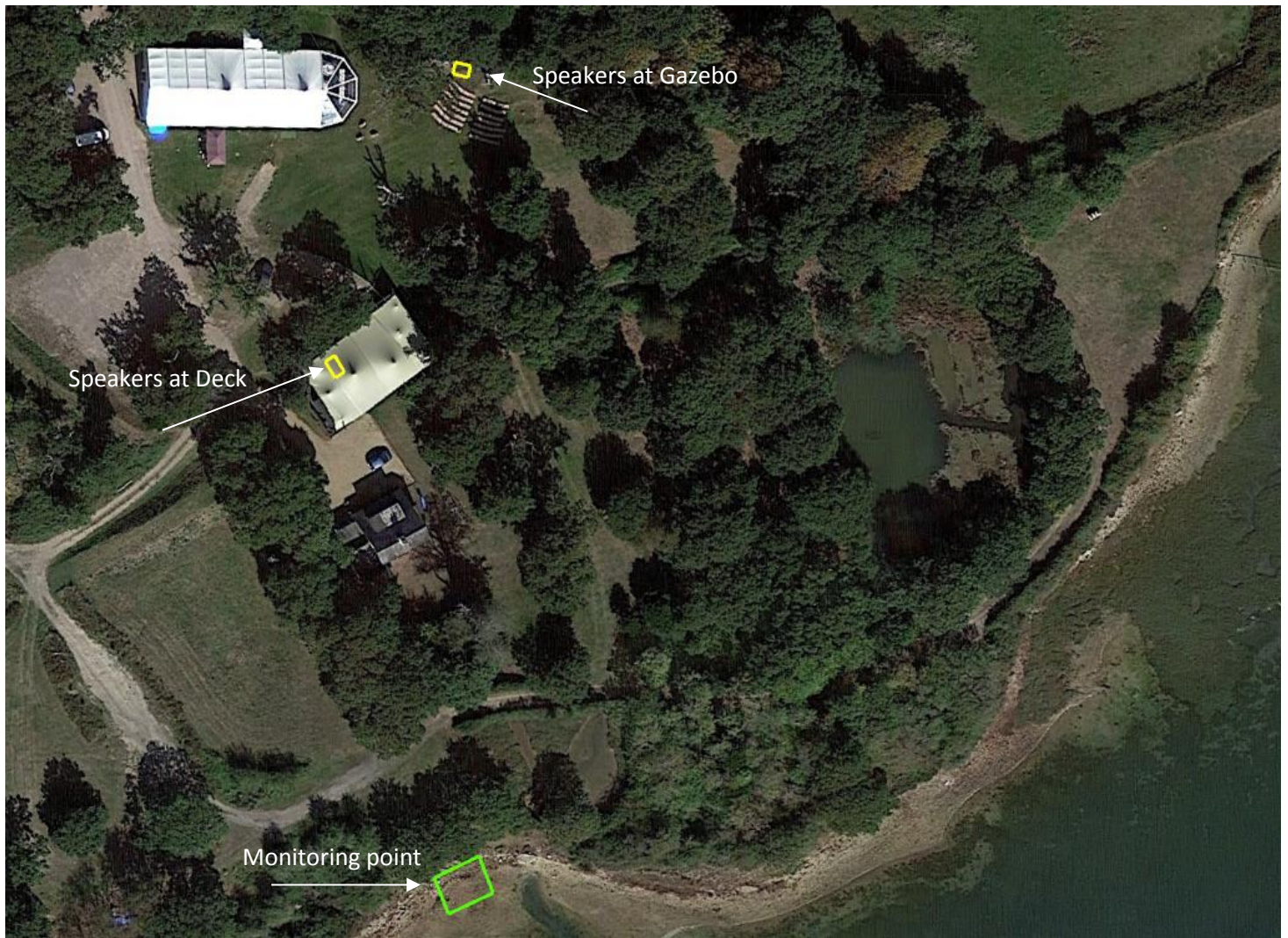
Fig B: Site closeup showing Marquee, Deck, Gazebo, siting of external speakers and external noise foreshore monitoring point in line of sound travel towards nearest residential receptors.
