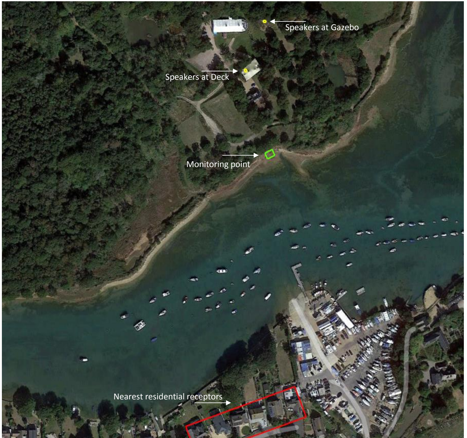
Fig A: Site overview showing Marquee, Deck, Gazebo, nearest residential receptors, siting of external speakers and external noise foreshore monitoring point in line of sound travel towards nearest residential receptors.
