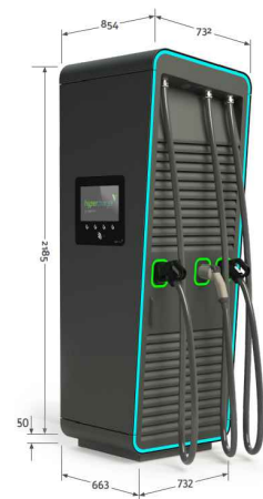
3D VIEW OF PROPOSED CHARGING EQUIPMENT | 1:50
