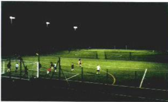
Image of a floodlit pitch demonstrating how the light is directed onto the playing surface whilst avoiding light spill and pollution.
