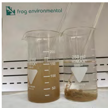
C. Test 3 Control vs WL 494 / 360 (further 15 second agitation from Test 2 plus 60 second settlement)
