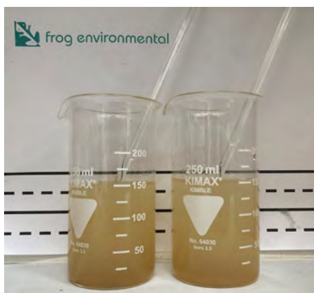
D. Test 1 Control vs WL 494 / 360 (15 seconds agitation plus 30 seconds settlement)
