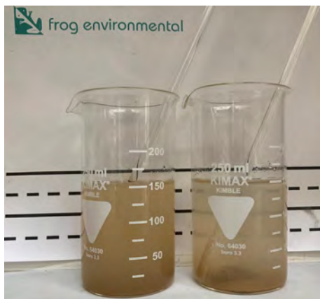
A. Test 1 Control vs WL 494 / 360 (15 seconds agitation plus 30 seconds settlement)
