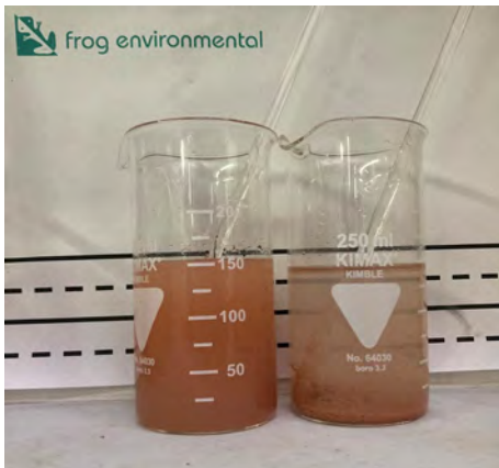
G. Test 1 Control vs WL 494 / 360 (15 seconds agitation plus 30 seconds settlement)
