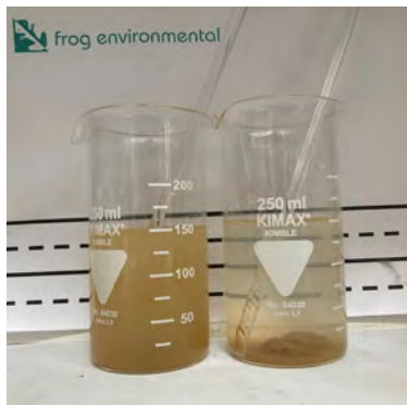
F. Test 3 Control vs WL 494 / 360 (further 15 second agitation from Test 2 plus 60 second settlement)
