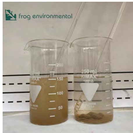
B. Test 2 Control vs WL 494 / 360 (further 15 second agitation from Test 1 plus 60 seconds settlement)
