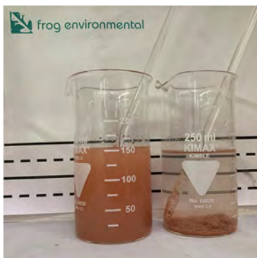
I. Test 3 Control vs WL 494 / 360 (further 15 second agitation from Test 2 plus 60 second settlement)
