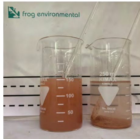
H. Test 2 Control vs WL 494 / 360 (further 15 second agitation from Test 1 plus 60 seconds settlement)
