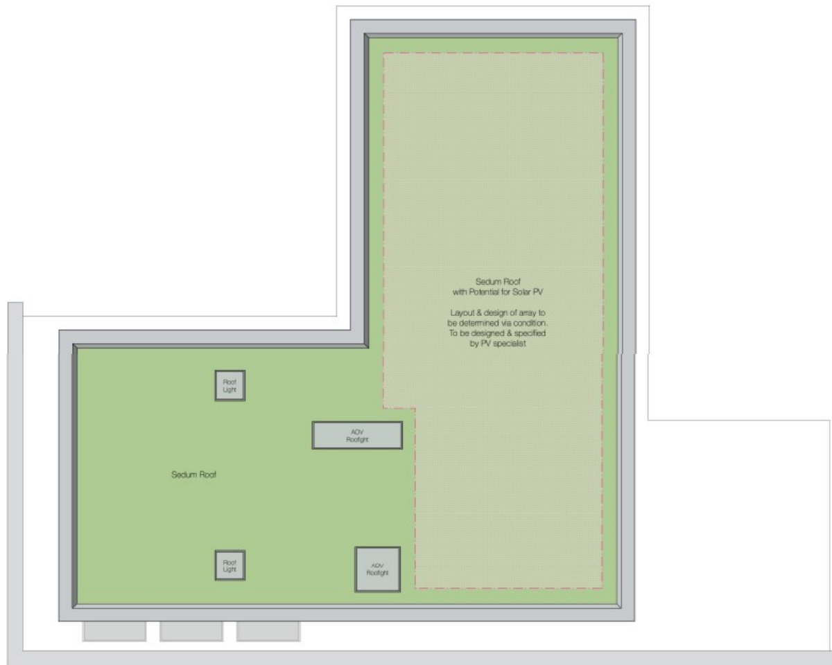
Figure 3: Illustration of PV layout location (Marlow Architects)
