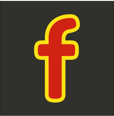
High Level flexbox Painted RAL 7022 Internally illuminated. 2500 x 2500mm Scale 1:50
