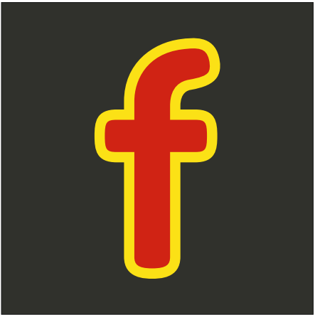
High Level flexbox Painted RAL 7022 Internally illuminated. 1450 x 1450mm Scale 1:25
