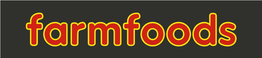
2no. New flexboxes Painted RAL 7022 Internally illuminated. 5800 x 1300mm Scale 1:50
