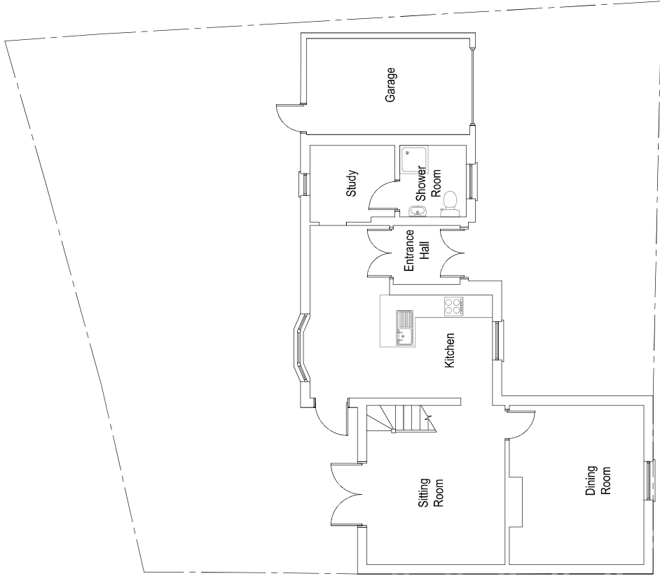
Existing Ground Floor Plan Scale 1:50
