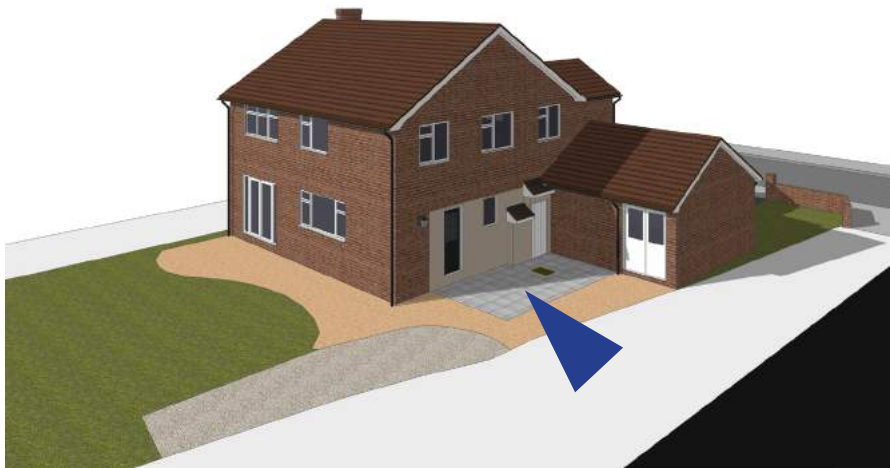
Above / 3D of the existing house from the rear. Area behind garage highlighted as underused space and possible location for an extension with no adverse impact on neighbours or surroundings.
