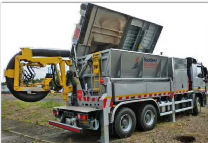
Figure 17. Large Vacuum Excavator
