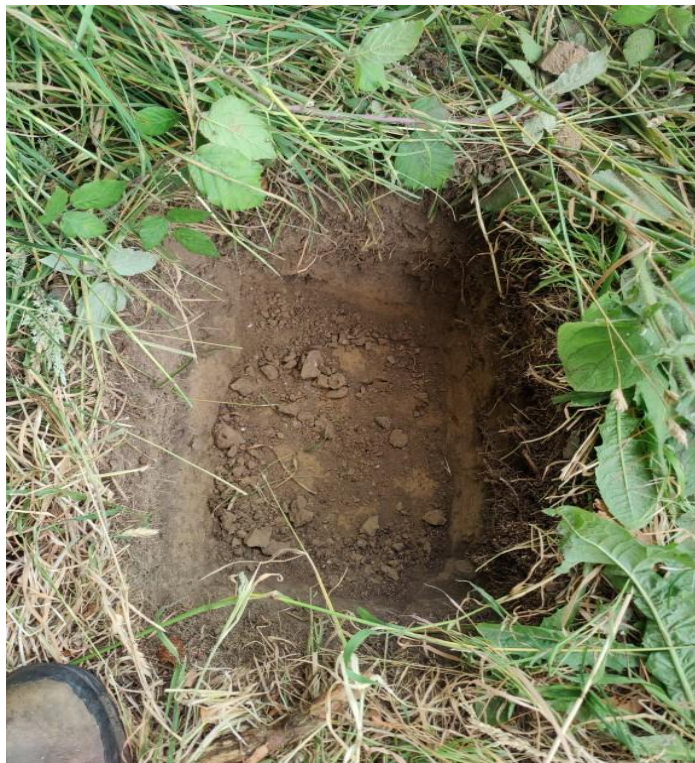
Photograph 11- Trial pit 3 extent. Ceased digging at 400mm in depth, as no further roots encountered.
