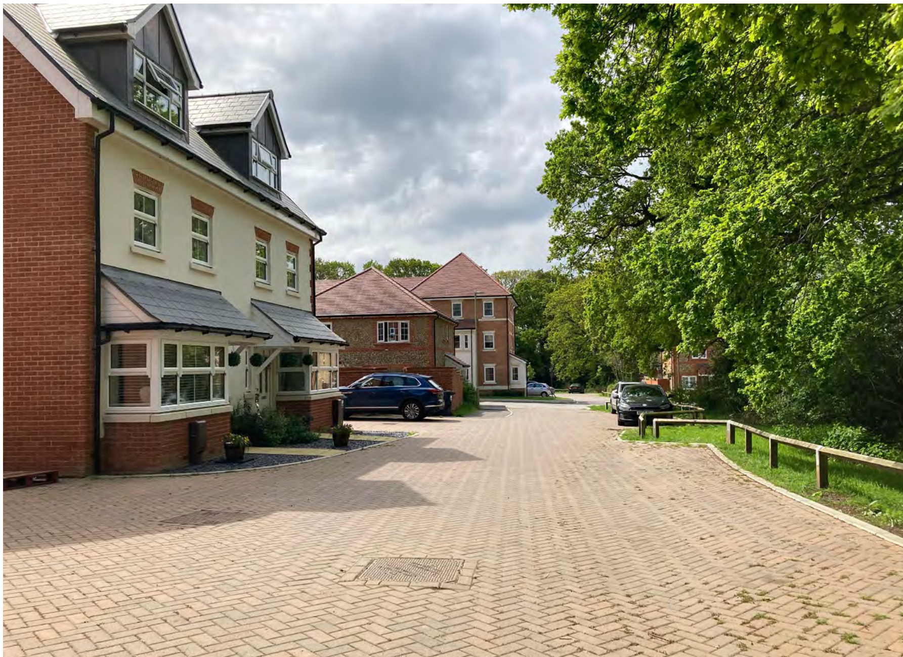
Use of block paved shared space parking lane at Catherington Park
