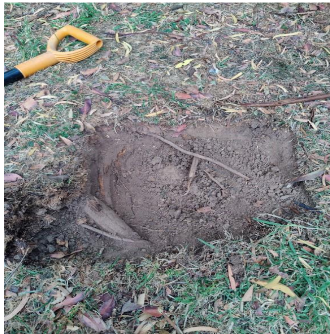
Photograph 7- Trial Pit 2: Immediately encountered a large root from Cider gum (T15) of 35mm in diameter, identified by its smoothness of outer root as opposed to the shaggy outer of Snow Gum (T16). Digging ceased at 100mm in depth due to the presence of large root.
