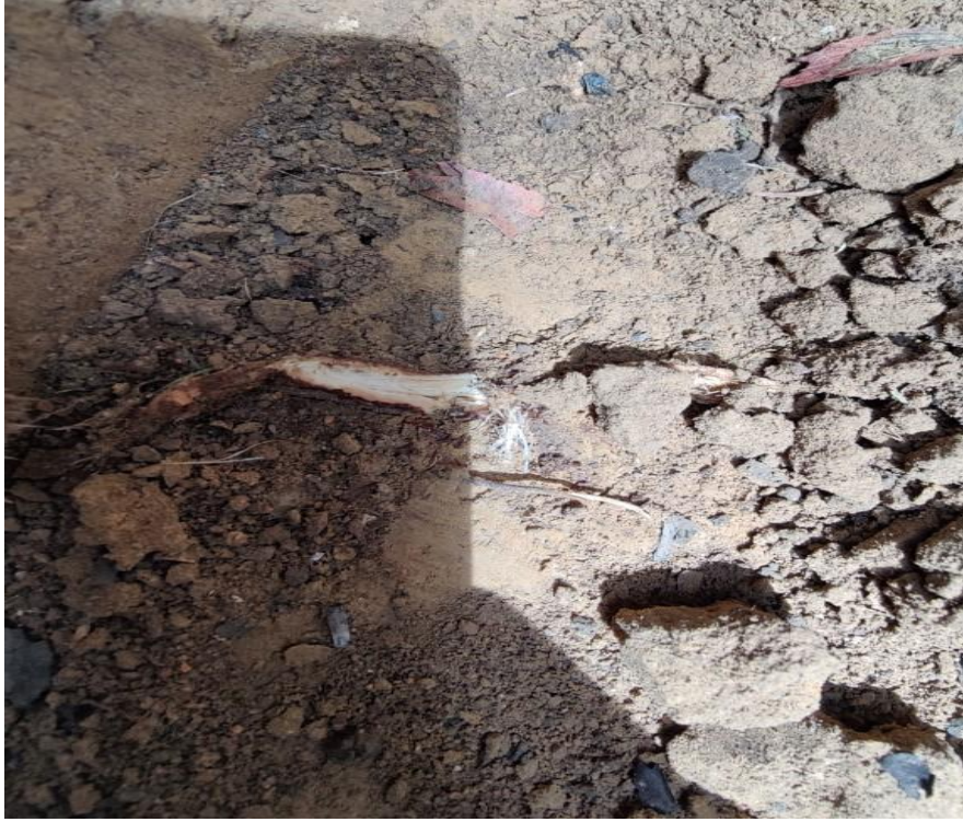
Photograph 5- Trial pit 1: At 450mm in depth one 10mm diameter root encountered- digging ceased due to denseness and dryness of the clay substrate.
