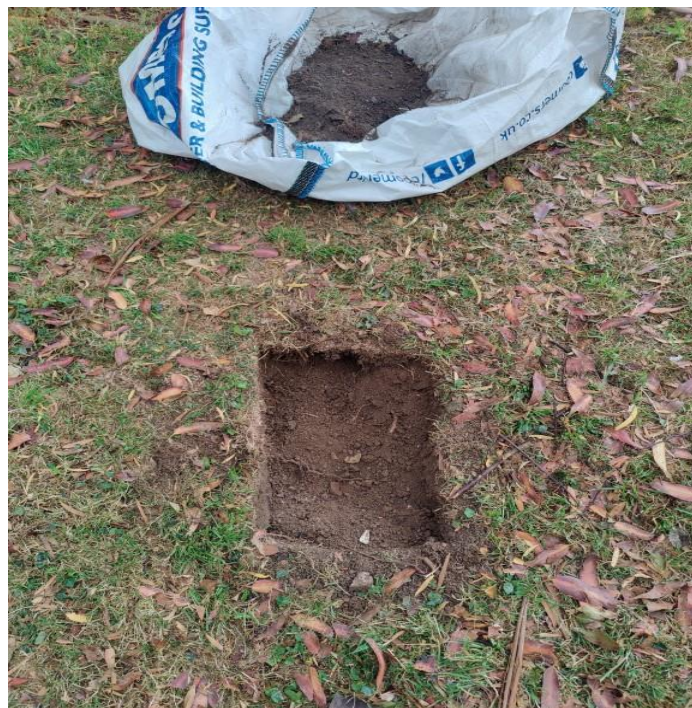
Photograph 2: Trial pit 1: commencement- only fibrous roots found at 50mm in depth. All pits to approximately 250mm x 400mm
