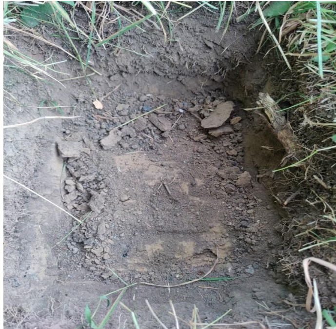
Photograph 10- Trial pit 3: 200mm in depth and due to the density of the clay a root of 15mm diameter was severed at 150mm deep. This was cleanly severed using a Silky Gomato. Note its location immediately adjacent to and running alongside the tennis court
