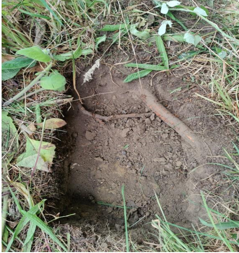
Photograph 14- Trial pit 4: Extent of dig depth of 300mm.
