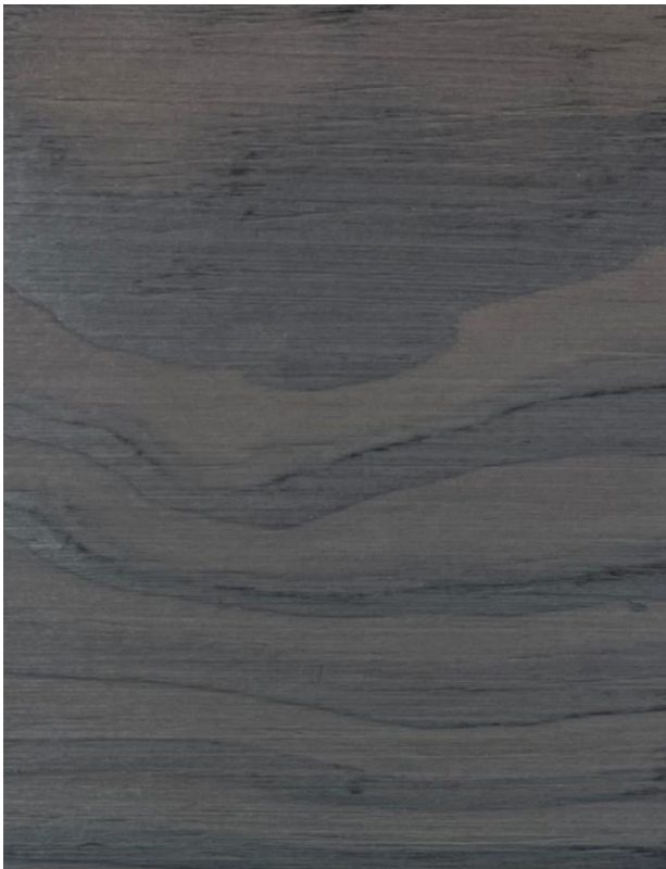
Figure 3: SHOU-SUGI-BAN – Charred Accoya Cladding in Anthracite grey
