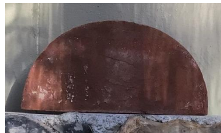
Figure 3: Curved brick Sample.
