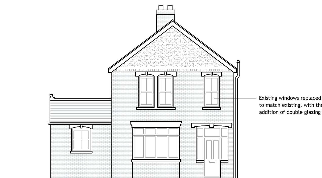
FRONT ELEVATION [North] 1:100
