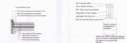
17 PROPOSED FOUNDATION DETAIL 1:25
