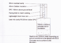
18 PROPOSED FOUNDATION DETAIL 1:25
