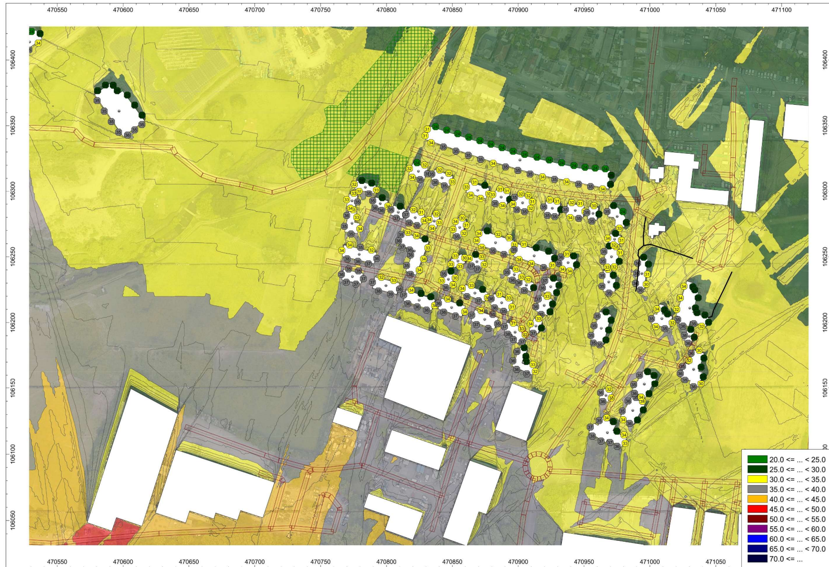
Figure C.3 – Predicted specific noise levels (dB L Aeq ) – all plant operating simultaneously/full capacity – NSR 1
