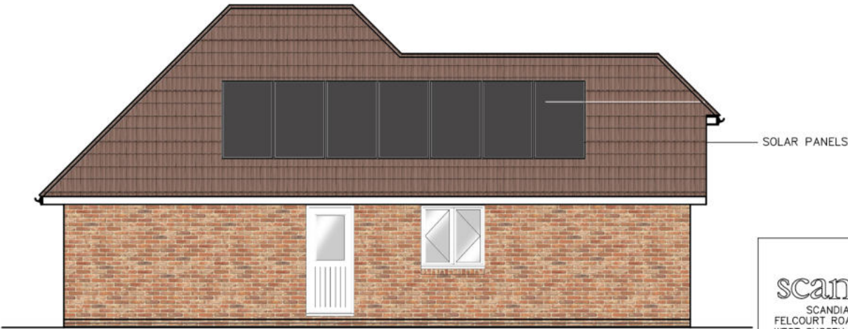
SIDE ELEVATION (SOUTH EAST)
