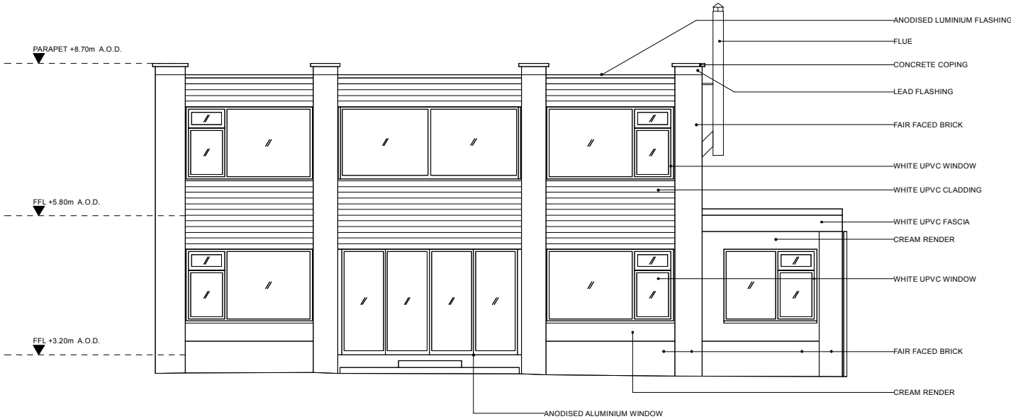
04. NORTH ELEVATION - EXISTING
