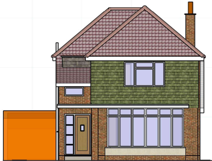
EXISTING SOUTH ELEVATION
