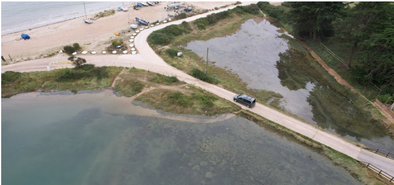
Fig 47: Source: TWE drone photograph of single vehicle width 44 meter section of HISC access road, water surrounds this on either side during high tides. This access road is not lit at night.
