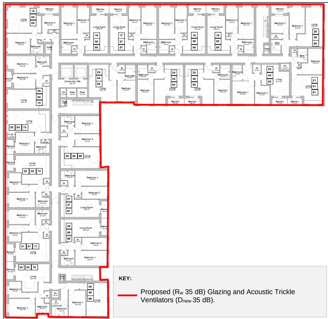
Figure 5.1: Acoustic Performance Recommendations
