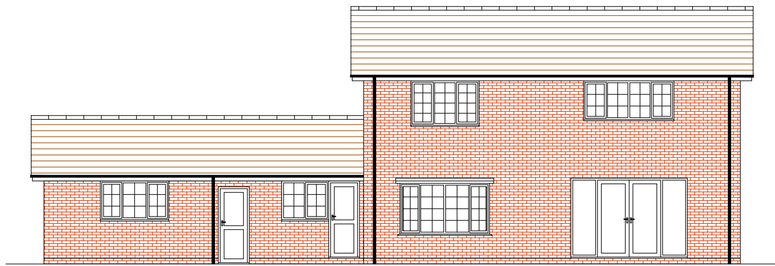
Existing South Elevation (1:100)
