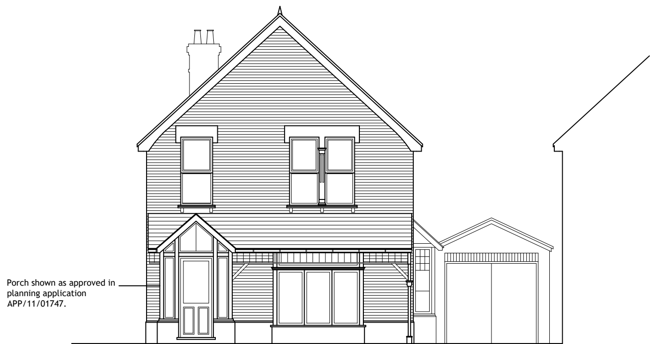
FRONT ELEVATION [west] 1:100
