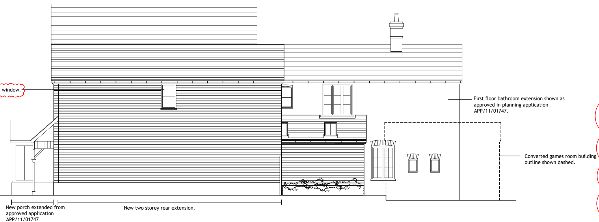
SIDE ELEVATION [north] 1:100
