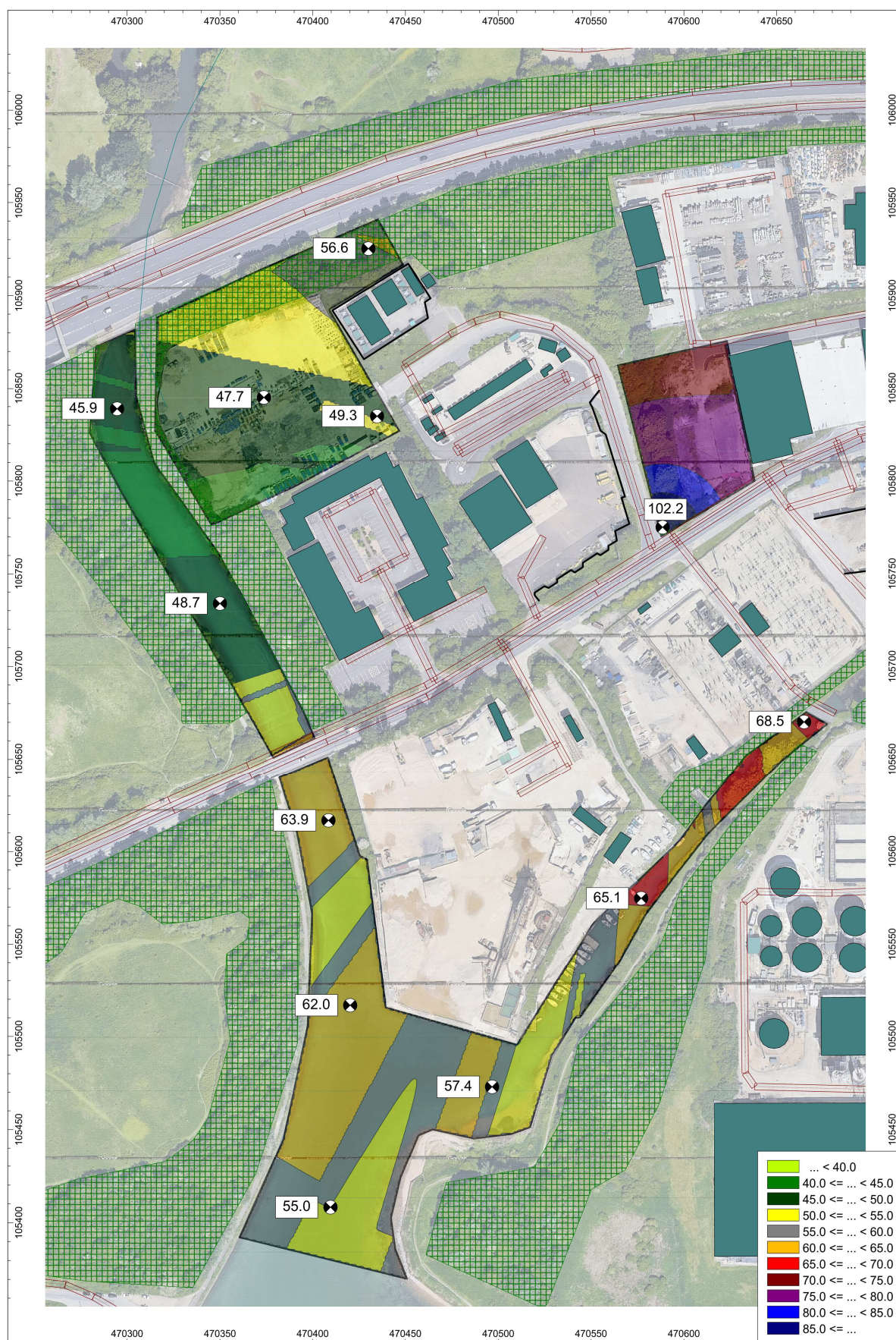
Figure B.5 – Predicted L_{Aeq} noise emissions – grid height of 4m – single source operating at 119 dB L_{WA}
