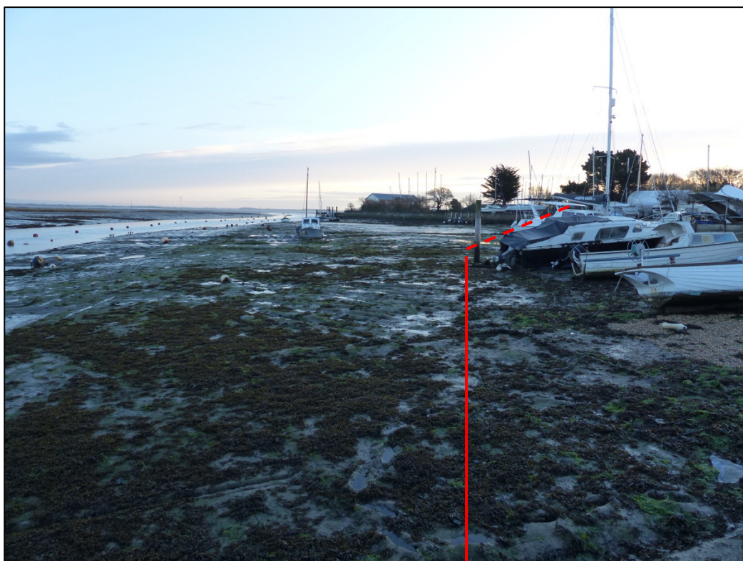
Figure 1: View across intertidal habitat, with red solid and dashed line depicting approximate location of new pontoon. All existing boats and other materials will be removed from the intertidal, with new berths situated on the seaward side of new pontoon.
