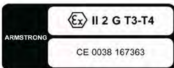
Figure 6: Indication sticker explosion safety
