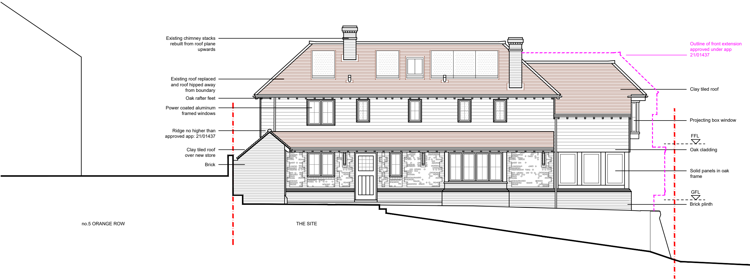
SIDE ELEVATION [west] 1:100
