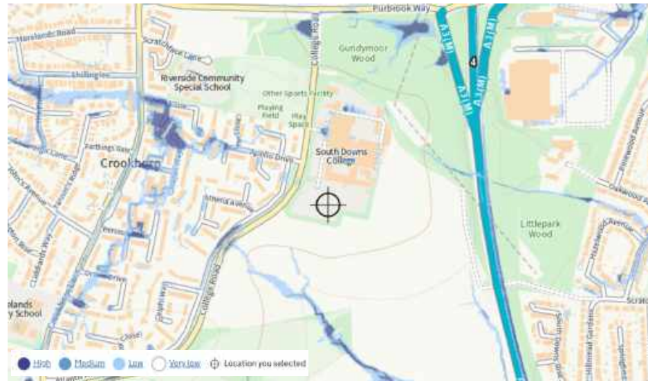
Figure 2.3 – Flood Risk from Surface Water
