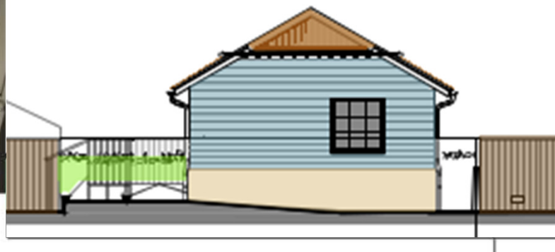
MACHINE MADE BRICK WITH AN APPEARANCE OF A RECLAIMED TRADITIONAL BRICK - TUMBLED DISTRESSED FACE. HOSKINS OLD FARMHOUSE BLEND OR SIMILAR
