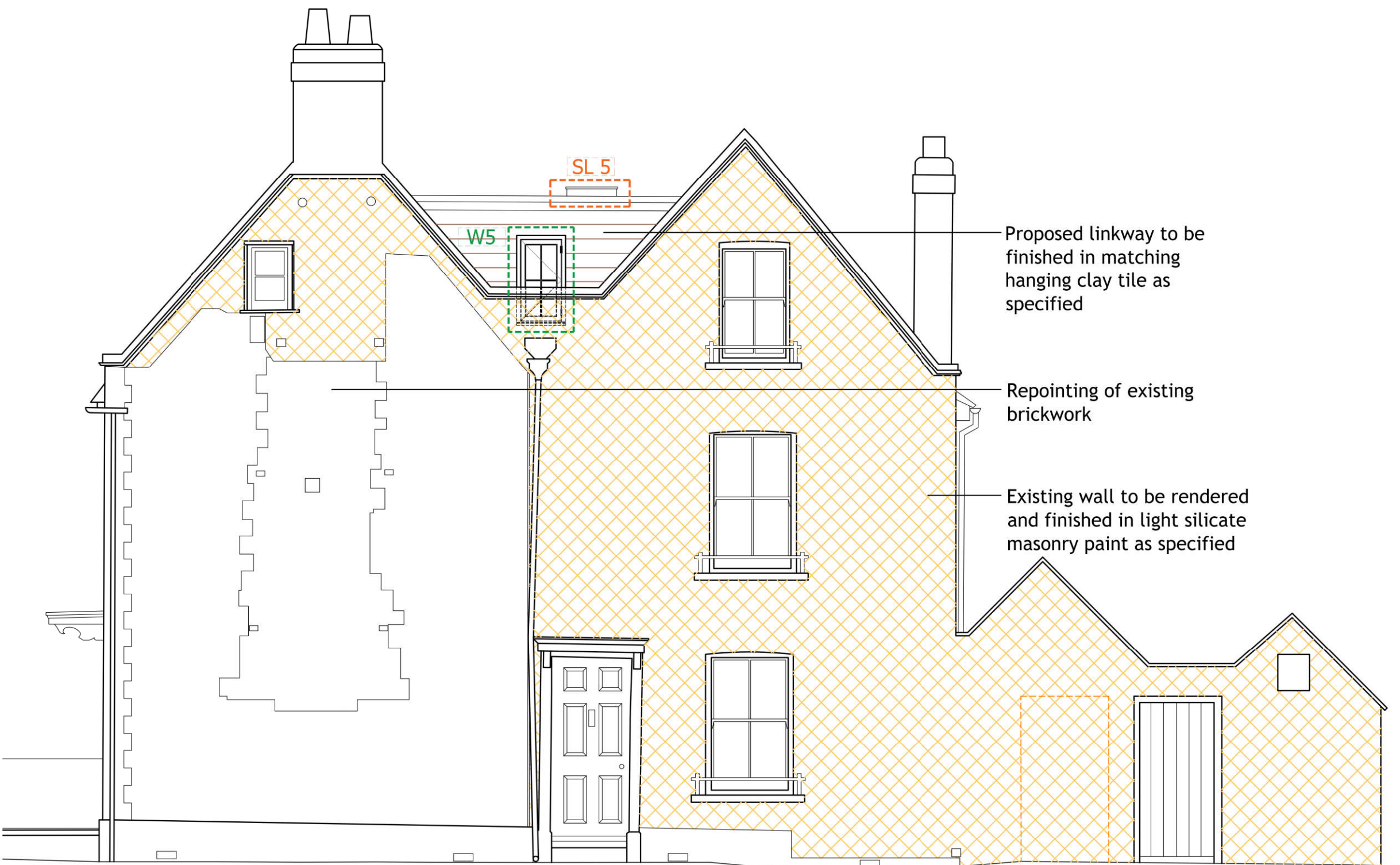
SOUTH WEST ELEVATION 1:50
