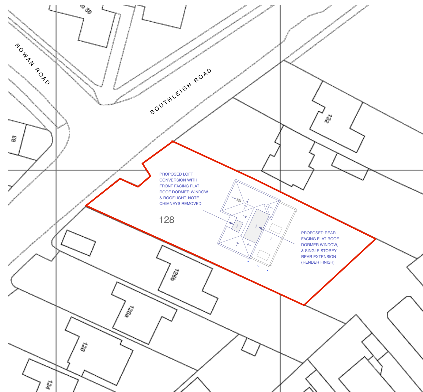
Proposed Site Plan at 1:500 scale
