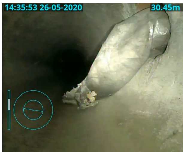
Pipework shows areas of POTENTIAL BLOCKAGE otherwise clear (or light silt)
